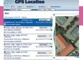
where and if they have stopped on the way. You also have the option to define areas ("electronic fence ") on a map where vehicles can or cannot move inside or outside. An alarm activates informing the responsible when a vehicle crosses the boundaries.
